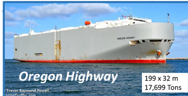
Figure 3: The M/V Oregon Highway the spectrum from which was measured by a bottom hydrophone located about 100 km south of Cape Cod in March 2017. The vessel is moving about 14 knots, and these data are from the closest point of approach (CPA) from the sensor, which is about 500 m.
